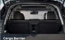
Cargo Barrier protects vehicle occupants from any loose items during sudden braking. Maximum load mass of 60kg.
